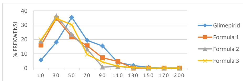
Figure 1. Particle Size Distribution Comparison Curve
