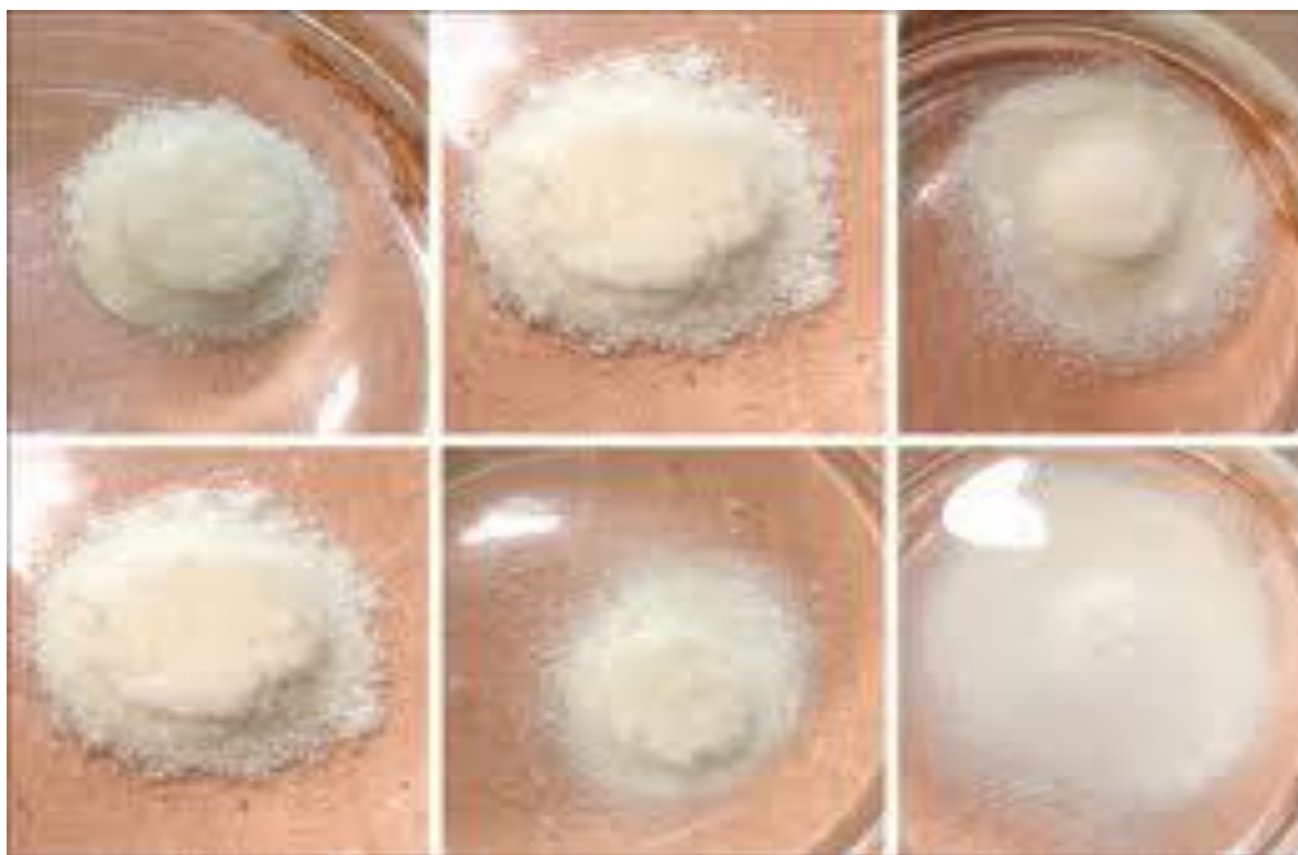
Fig. 15 Disintegration of tablet in 5,10,15,20,25,30 min respectively
