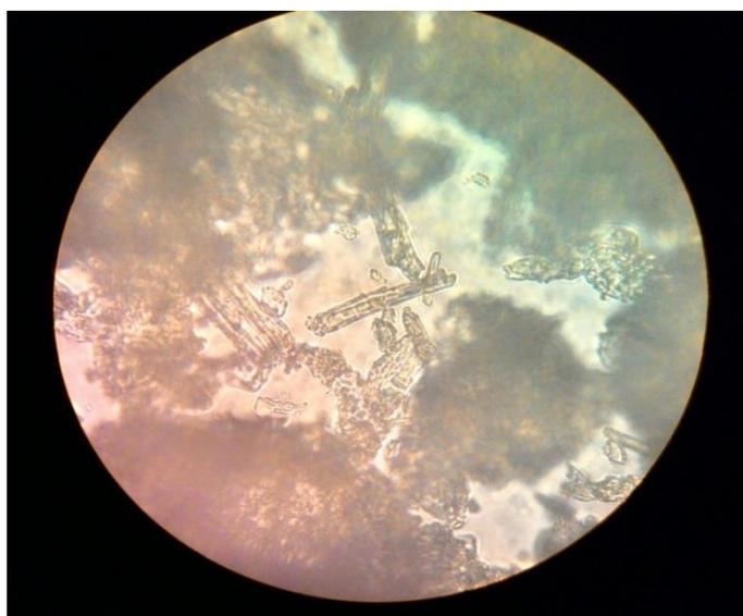
Figure 4: Microscopic photo of microcrystalline cellulose (MCC) from rice straw
